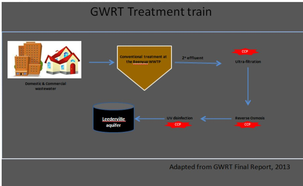
**Figure 2:** Beenyup Groundwater Replenishment Trial treatment train.
